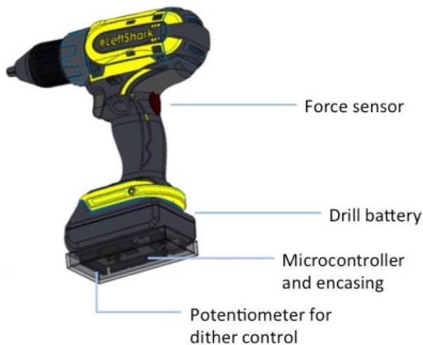
Figure 8: Future design iteration that emphasizes portability. Arduino or similar microcontroller and electronics are attached on outside of drill and in protective casing.
