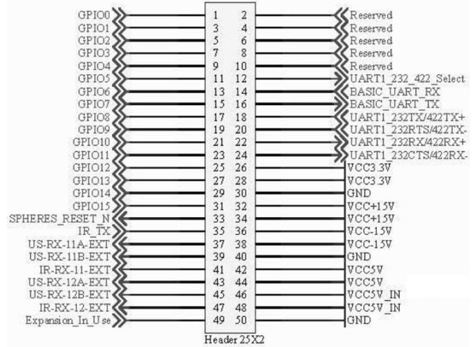
Fig. 14. SPHERES expansion port electrical interface pin assignments.
